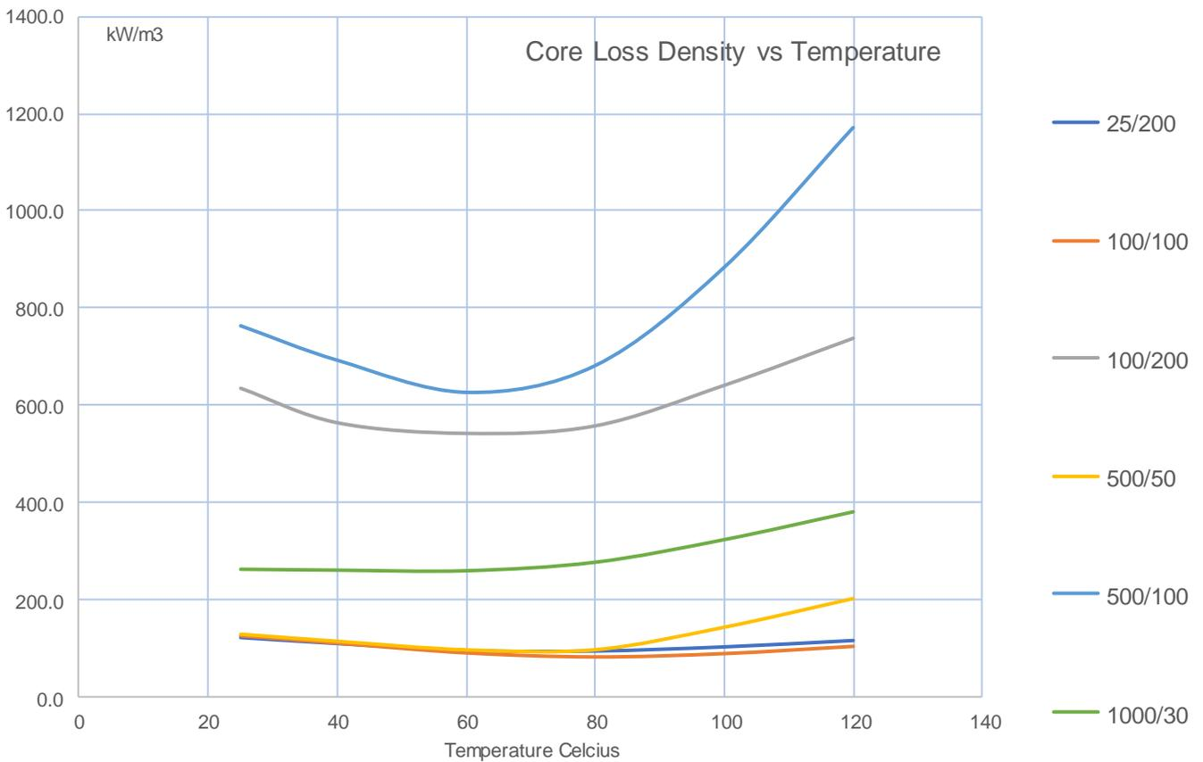
CORE LOSS VS TEMPERATURE SAMPLE COMPARISON HF03 (T29-19-15) 3f36 (ETD 34)
