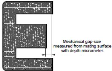
1 CORE GAP - One with Gap and One with no gap
