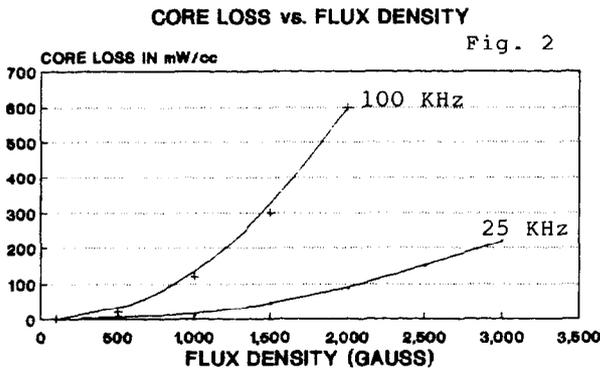
tially. To reduce the core loss, the flux density could be reduced by choosing a core with a larger cross sectional area. This option affects size, weight and cost. The flux density can also be reduced by operating at a higher frequency or increasing the number of turns on the coil. These options trade improvements to hysteresis losses for higher eddy current losses and higher copper losses. The total power loss may even increase with such trade-offs.
