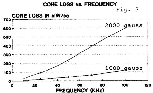
The following formula can be used to approximate core loss of Ferrite International's power materials at gauss levels and frequencies other than those published.
