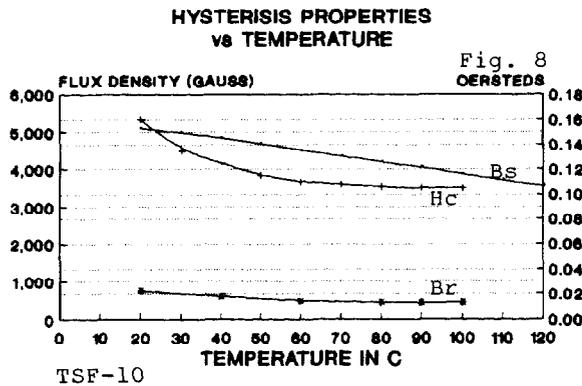
power transformers and output inductors to operate at flux densities below saturation at the highest temperature the cores will be exposed to.
