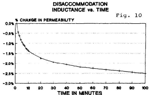
Mechanical stress due to excessive tension when winding toroids, excessive clamping pressure when assembling mated cores or pressure induced from coatings or glues can cause the initial permeability to decrease. The permeability remains decreased until the stress is removed.
