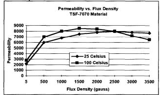
Permeability varies with flux density and temperature, hence the measured inductance also changes with changes in flux density and temperature. Therefore, the flux density and temperature must be controlled. To calculate the test voltage for a given flux density, the following formula is used: E = 4.44 f N B Ae  $10^{-8}$ f = frequency in Hz N = number of turns B = flux density in gauss Ae = effective core area in cm<sup>2</sup>
