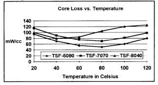
Core loss varies exponentially with changes in flux density. Therefore, samples must have uniform cross sectional areas throughout their magnetic path lengths. Measuring core loss on cores with non-uniform cross sectional areas is not accurate no matter if effective cross sectional areas are used or minimum cross sectional areas are used, because the flux density throughout the path length is not controlled.
