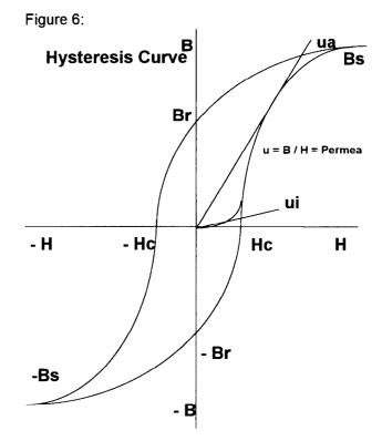
Saturation flux density (Bs) is a material's maximum magnetic induction. Saturation can be seen in quadrant 1 of the Hysteresis curve. When increases in magnetizing force (H) no longer cause significant increases in magnetic induction (B), the material is said to be saturated.
