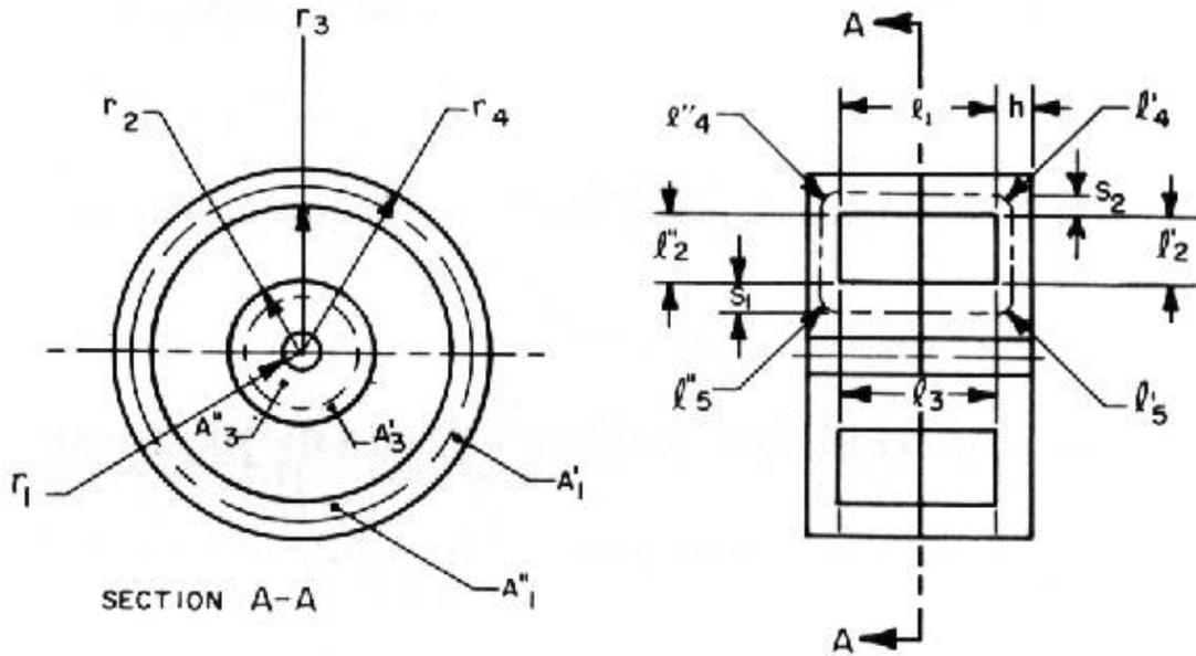
**FIGURE 6 POT CORE SET DIVIDED INTO 5 SECTIONS**
